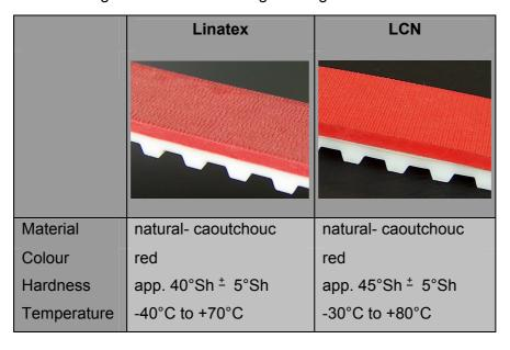
At Norditec LCN can be applied, as well as Linatex, by glue or seamless by vulcanisation.
